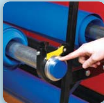
Aluminum safety collars, yellow security bars, blue vinyl end caps
